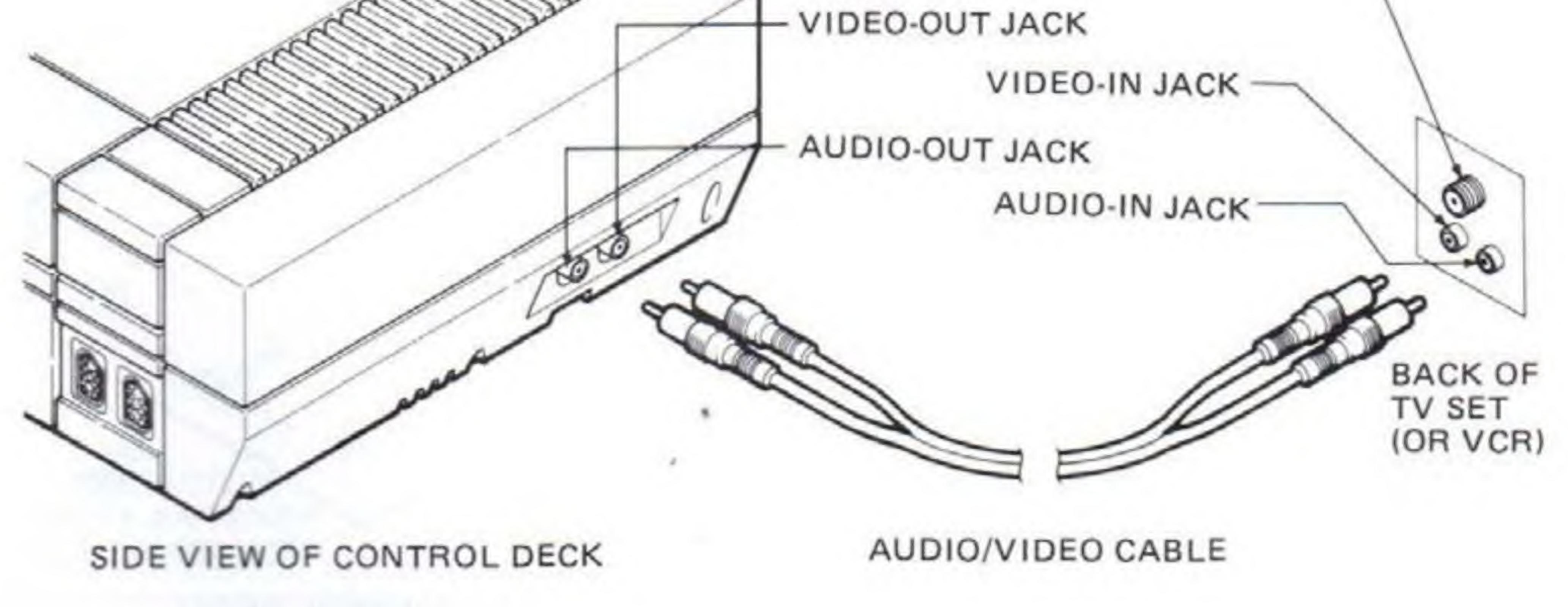
Note! Color coding of TV connections may differ from that of audio/video cable and Control Deck.
